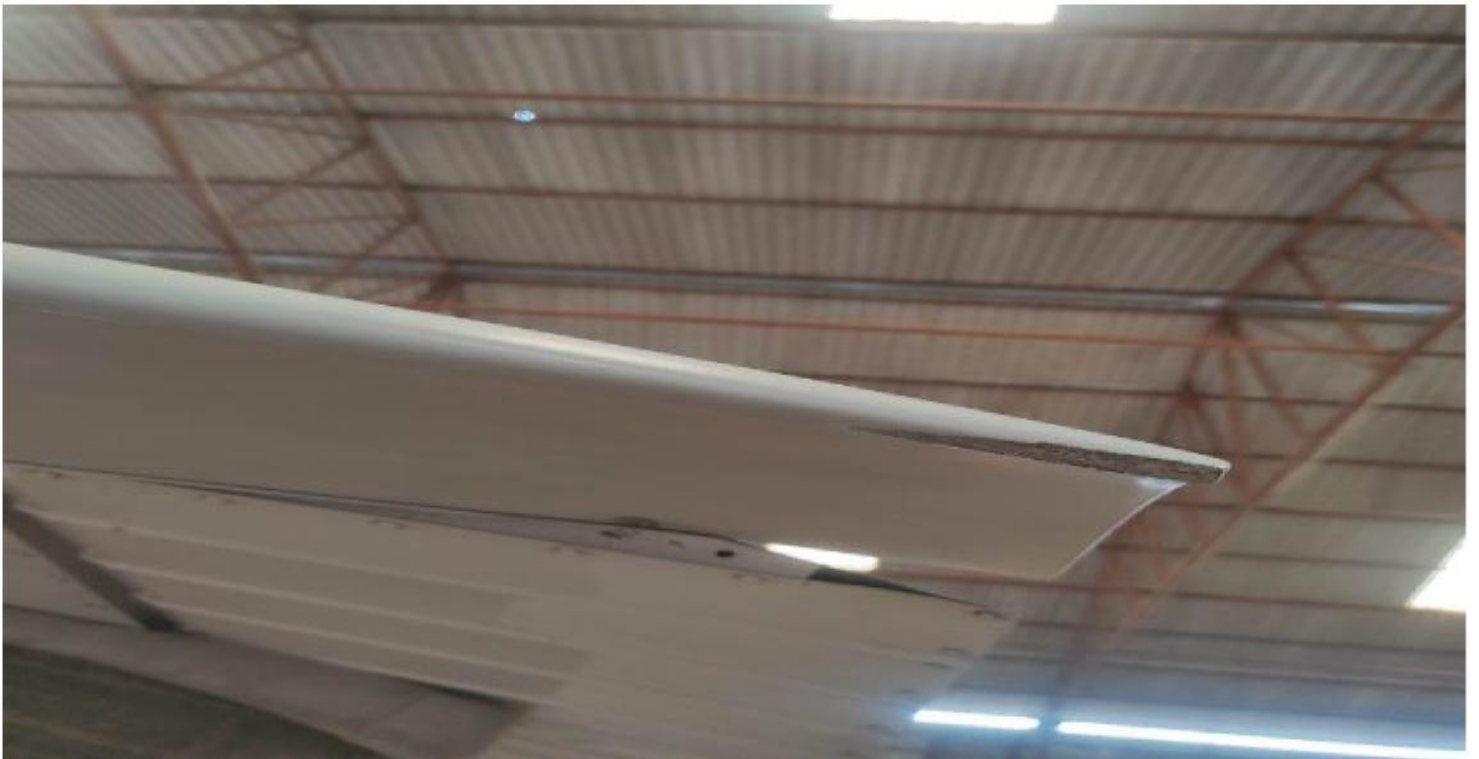
14- Tip Assy Wing LH (0523565-29) trailing edge corner found scratched.
